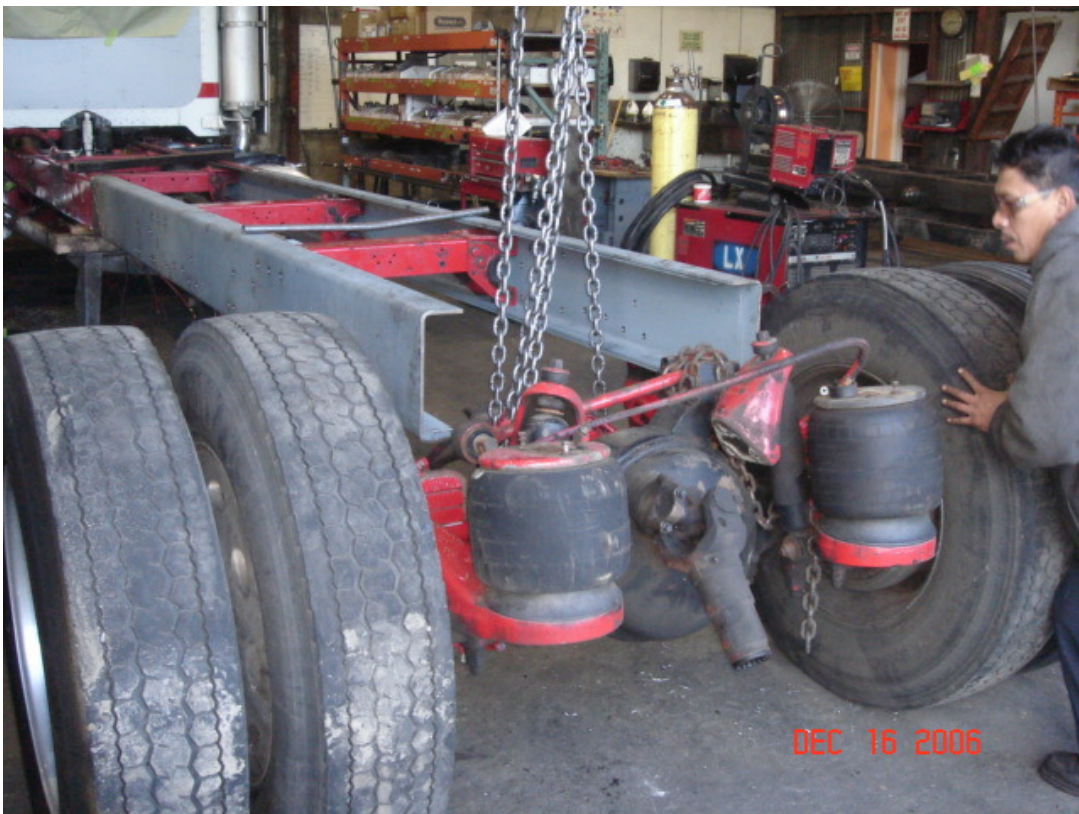
STEP # 4: Suspension is reinstalled. Drive lines stretched and modified for unit, if needed new brake cams will be installed or added when a single brake cam is present
