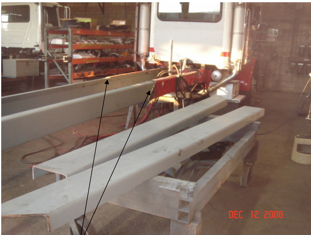
STEP # 2: Chassis is cut at 45 degree angle in one single location. New channels are designed specifically to fit current chassis design. New channel extension is welded at 45 degree angle for higher rigidity and structural strength.
