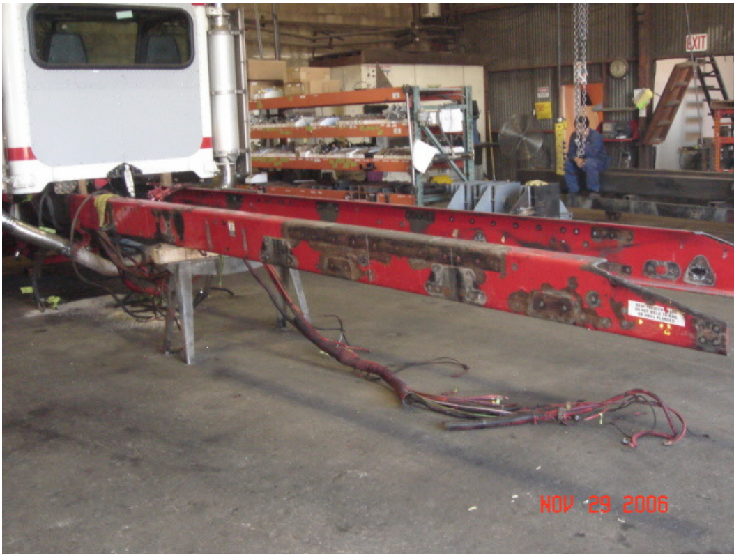
STEP # 1 :Unit is completely disassembled, all electrical air and hydraulic systems, suspensions and braking systems are removed.
