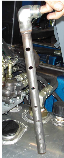
Figure 6. In-Flow hydraulic fluid pressure distribution manifold
