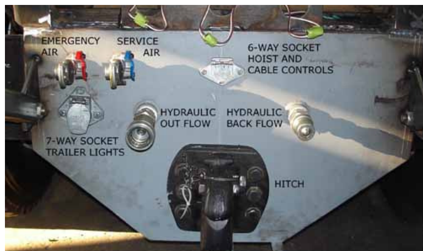
Figure 3. Hitch plate component identification
