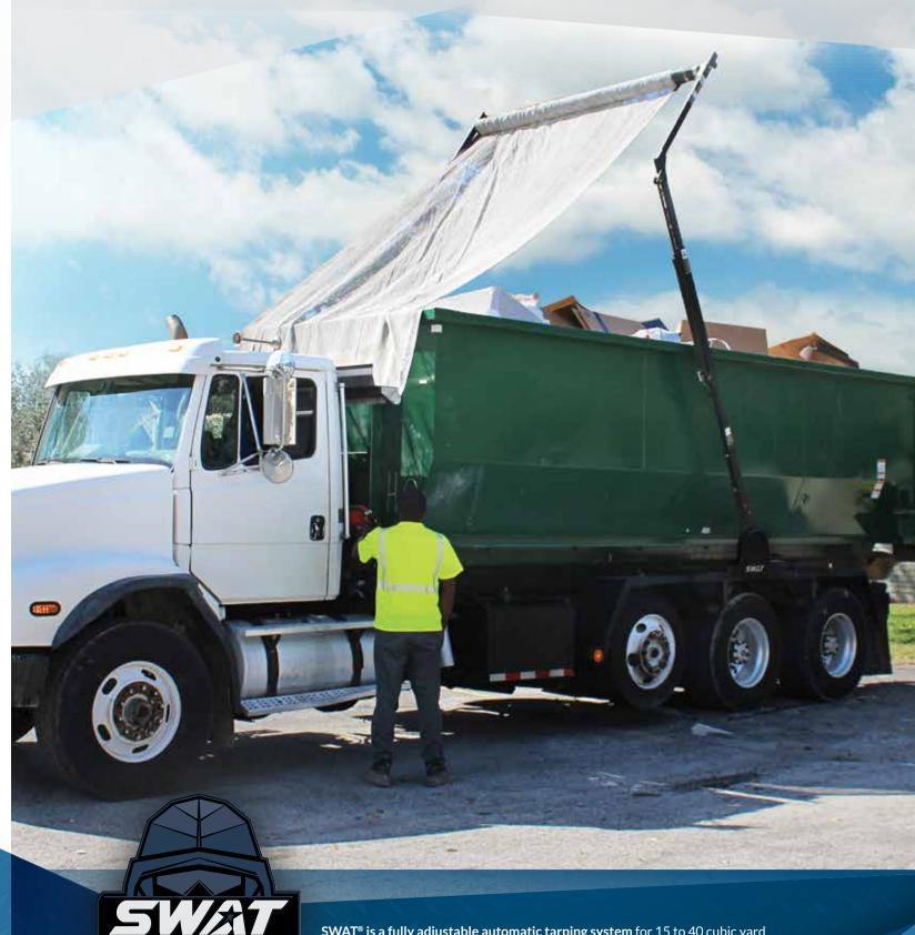
**SWAT®** is a fully adjustable automatic tarping system for 15 to 40 cubic yard containers. Designed with the end user in mind, the SWAT® was engineered to surpass all established technologies in the industry, thereby delivering maximum uptime and safety at a competitive price.
