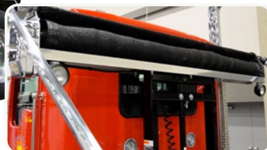
• Tower Rests at height of average 20yd container and extends 36" (Integrated Housing)
