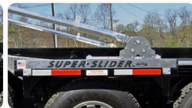
• Versatile pivot range with 180° arm rotation. Gear-driven spring pivot combined with patented sliding mechanism allows 20 in. of travel to easily accommodate 20-, 30- and 40-yd containers. Narrow profile (above) meets 108" outside mounting requirements when mounted on outside of fender.
