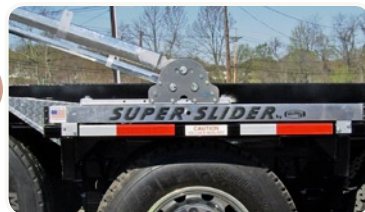
• Versatile pivot range with 180° arm rotation. Gear-driven spring pivot combined with patented sliding mechanism allows 20 in. of travel to easily accommodate 20-, 30- and 40-yd containers. Narrow profile (above) meets 108" outside mounting requirements when mounted on outside of fender.
