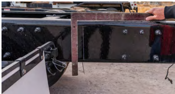
1. Vertical mark determination on chassis frame rail.
