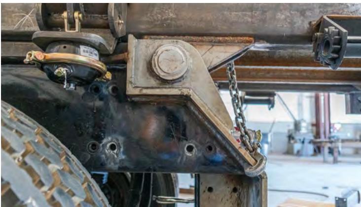
Left hand side full welded to apron.
