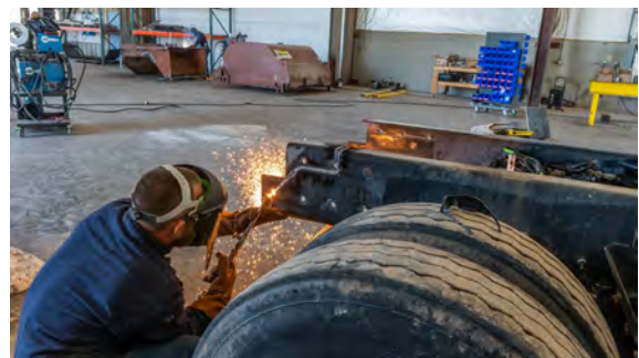
4. The removal of the excess chassis frame rail from the vertical and step mark determinations.
