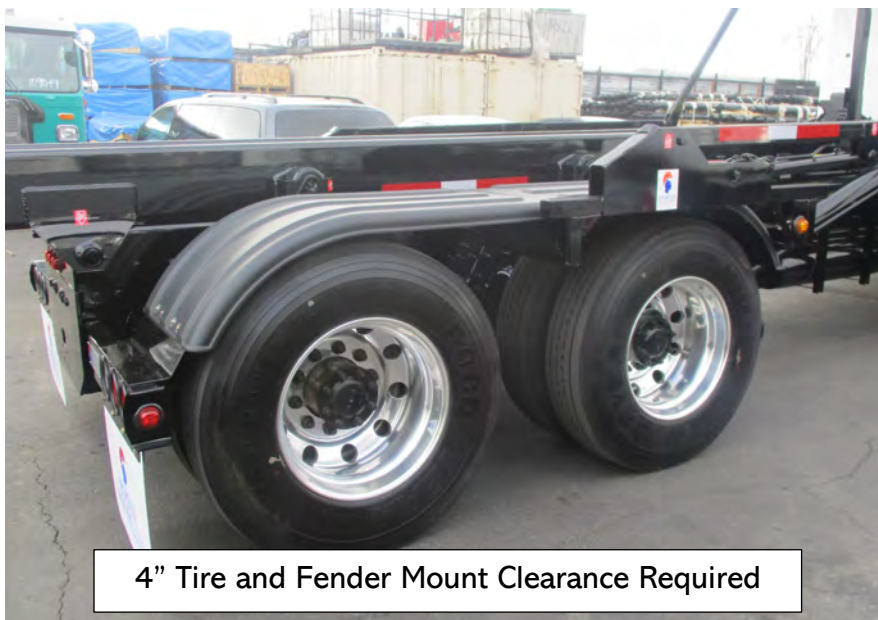
Full Length Plastic Fenders Example Figure
