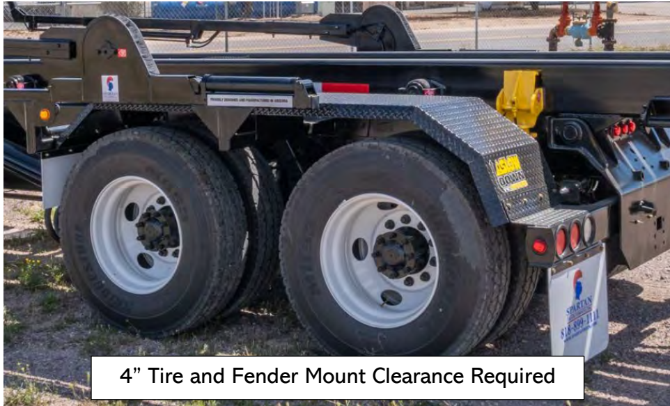
Full Length Steel Fenders Example Figure
