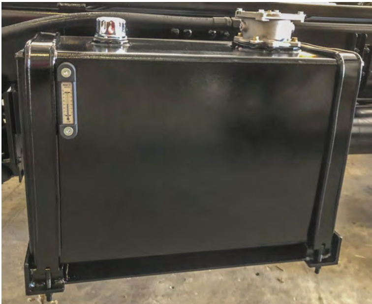
The Complete Hydraulic Tank Assembly
