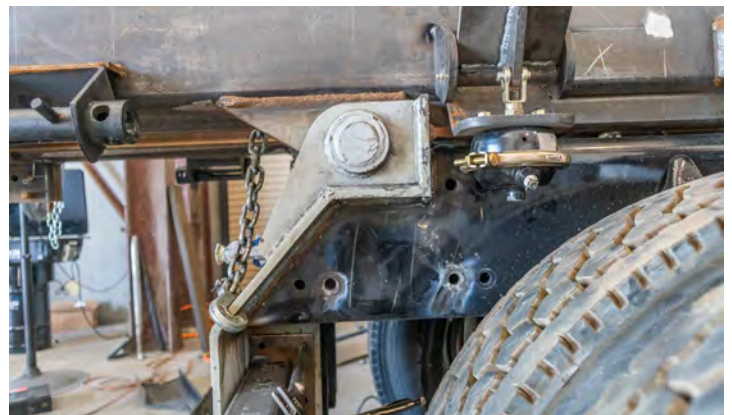
Right hand side full welded to apron.
