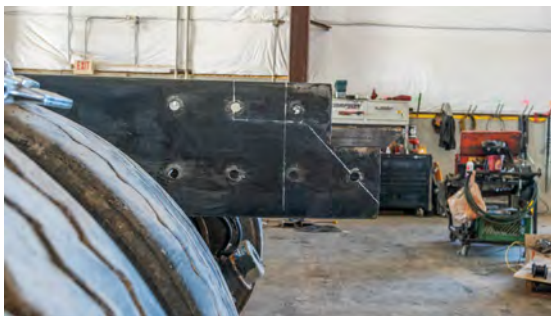
3. Vertical and step marks on chassis frame rail (existing roll off chassis).
