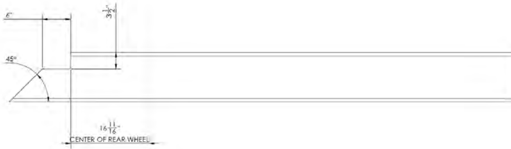
Chassis Frame Rail Cut-Off Measurement Diagram
