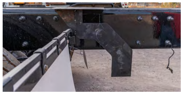
2. Step cut mark determination on chassis frame rail.
