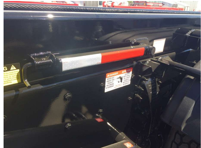
Safety Stand Securement - Spring Loaded Latch
