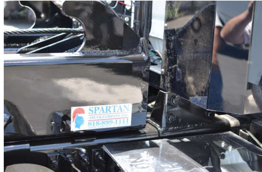
Safety Stand Securement - Spring Loaded Latch
